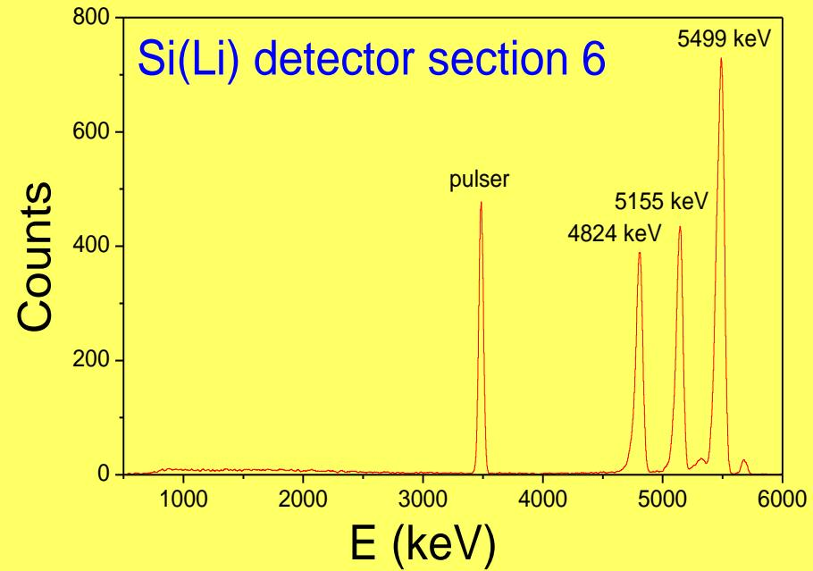
$\alpha$ - spectrum from pixel#6,  $T=22^\circ\text{C}$
