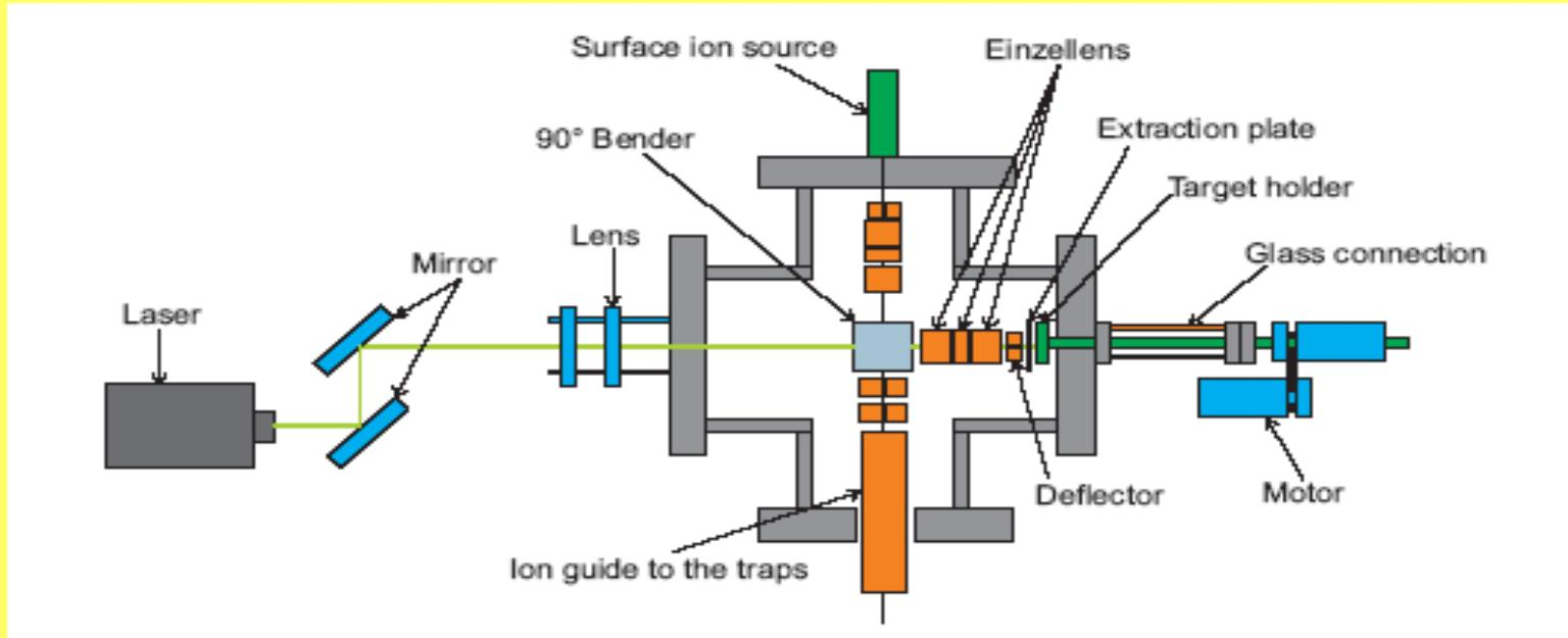
*Figure : Drawing of the ion source device for mass calibration by well known reference. A laser beam is focused on the rotatable target. The ions produced are removed with an extraction plate and directed to a 90°-bender by a deflector and by the Einzel lens (three electrodes: two of them with the length of 45 mm and one with the length of 15 mm installed with the  $\approx 1$  mm gap between each other). Ion guide is delivering the ions towards the traps.*
